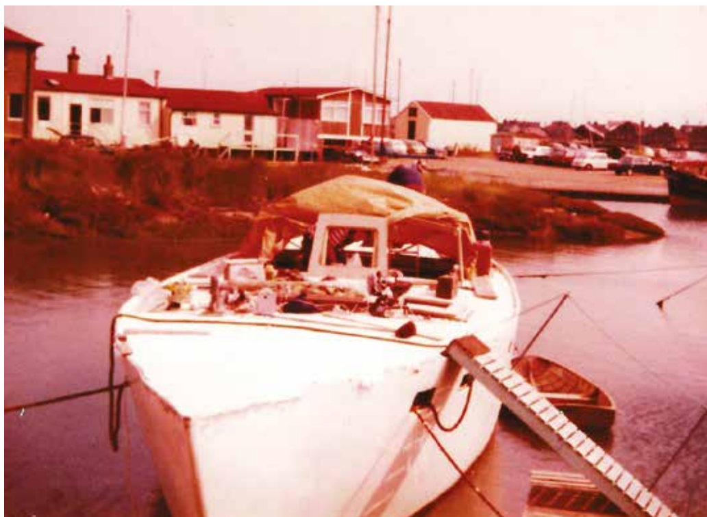
Building the wheelhouse after sheathing the deck with woven rovings GRP cloth
