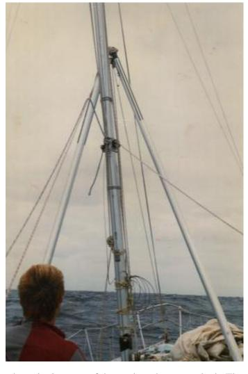
spotted that a cap shroud had hooked itself under the stripping arm of the starboard runner winch. That cleared and it was all over bar the shouting. With Haven winding, first to swing out the bi-pod to the vertical and then to complete the hoist with the crane line, and myself easing the steadying lines to maintain tension, our new mast rose until it was upright with the heel, guided by Paul and Cleater, poised over the deck ring.
