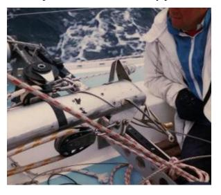
Paul sawed off the ragged broken butt end of our Mk II mast and fitted the original heel plug while Haven and I riveted on mast-bands and generally prepared the top of what had been a fractional rig mast, to accept its new role. Cleater backed up all round and had the presence of mind to keep
