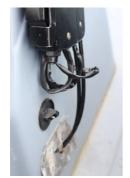
Check that the Anchor and Tow bridle are securely fitted. The Tow bridle should be inboard when not in use
