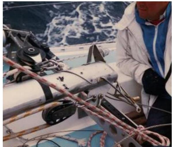
Paul sawed off the ragged broken butt end of our Mk II mast and fitted the original heel plug while Haven and I riveted on mast-bands and generally prepared the top of what had been a fractional rig mast, to accept its new role. Cleater backed up all round and had the presence of mind to keep
