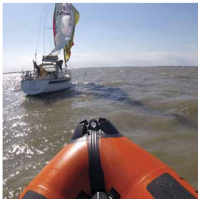
Yacht Meander with main and cruising chute jammed aloft
