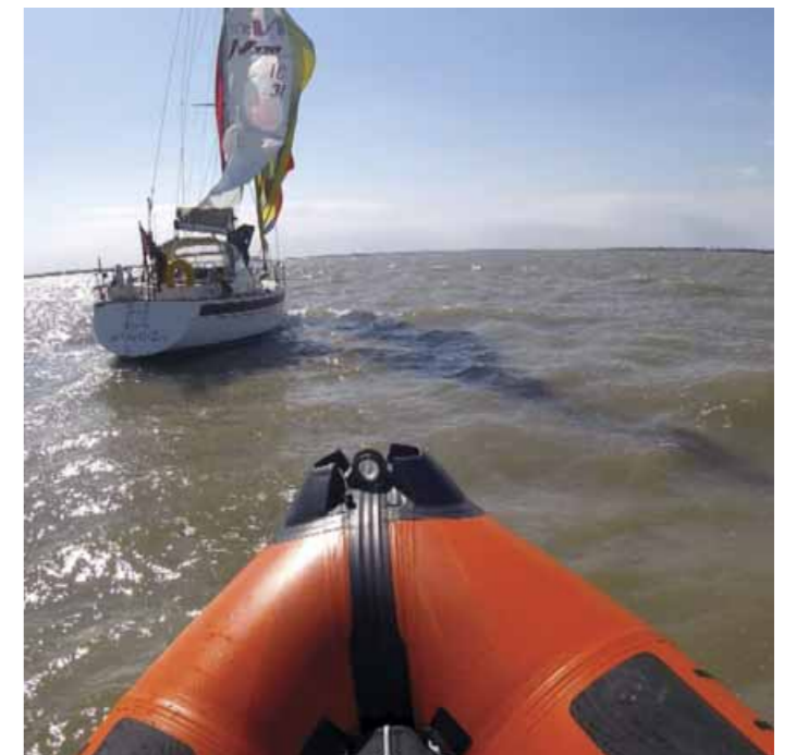
Yacht Meander with main and cruising chute jammed aloft
